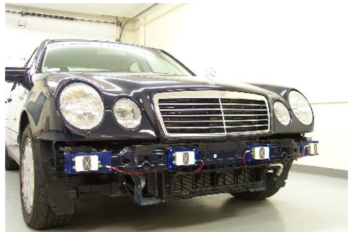
Mounting of the 24 GHz Short Range Radar System during testing
