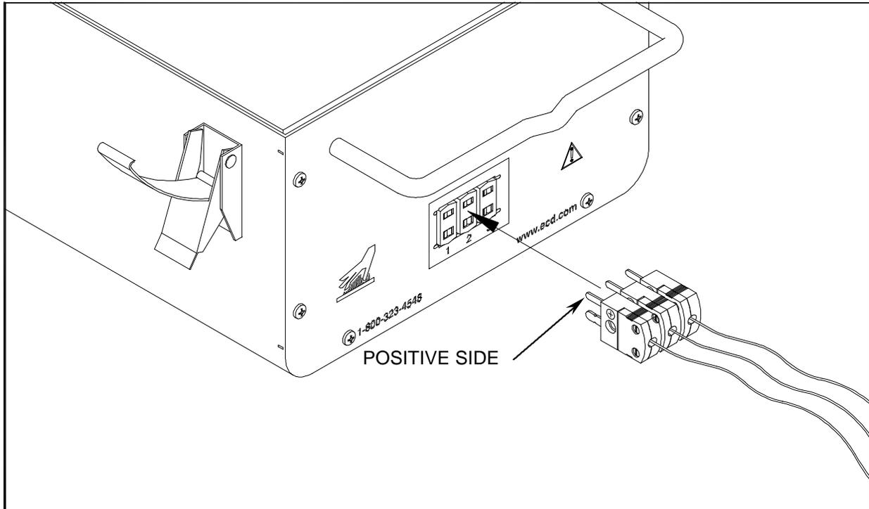
*Figure 4-6: Thermocouple Sensor Connection*
