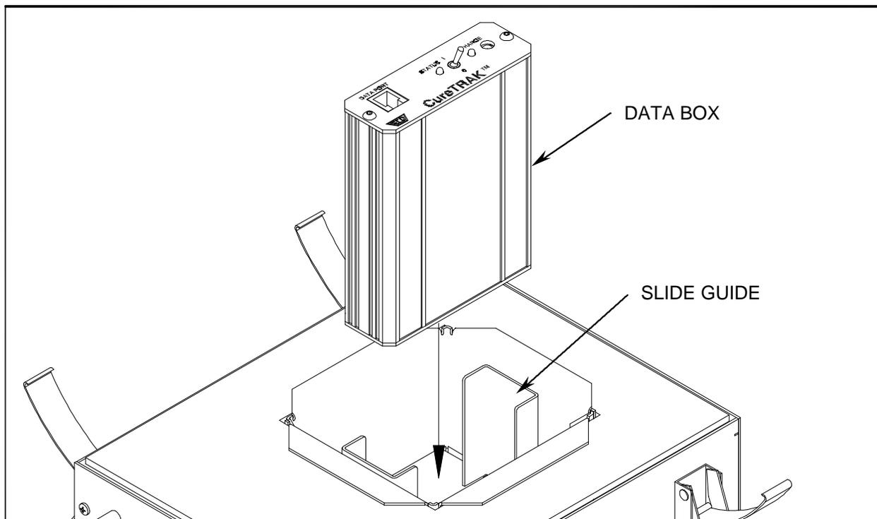
**Figure 4-1: Data Box Installation**
