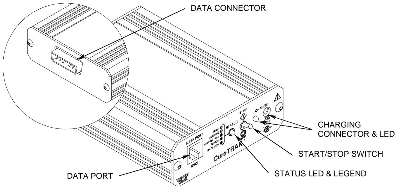
*Figure 2-4: Data Box Exterior Features*
