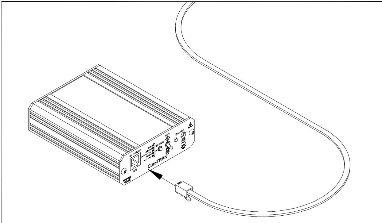
**Figure 4-10: Data Communication Connection**
