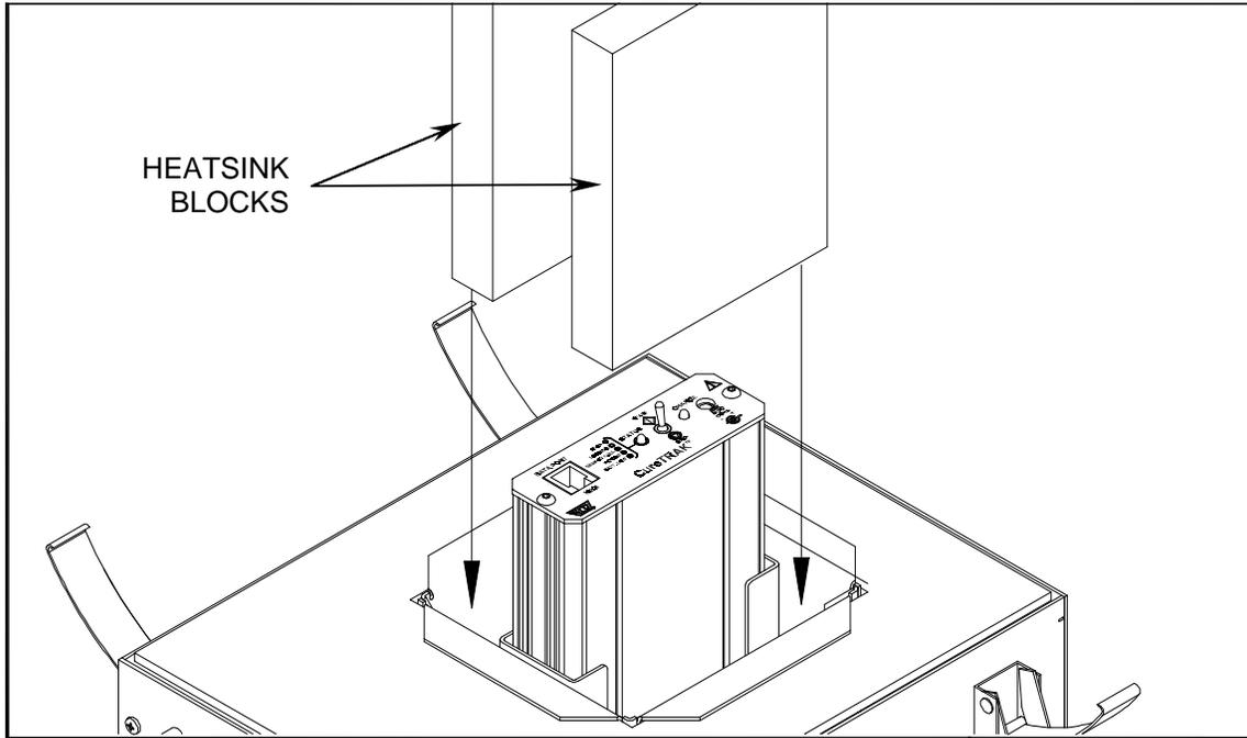
**Figure 4-4: Heatsink Blocks Insertion**
