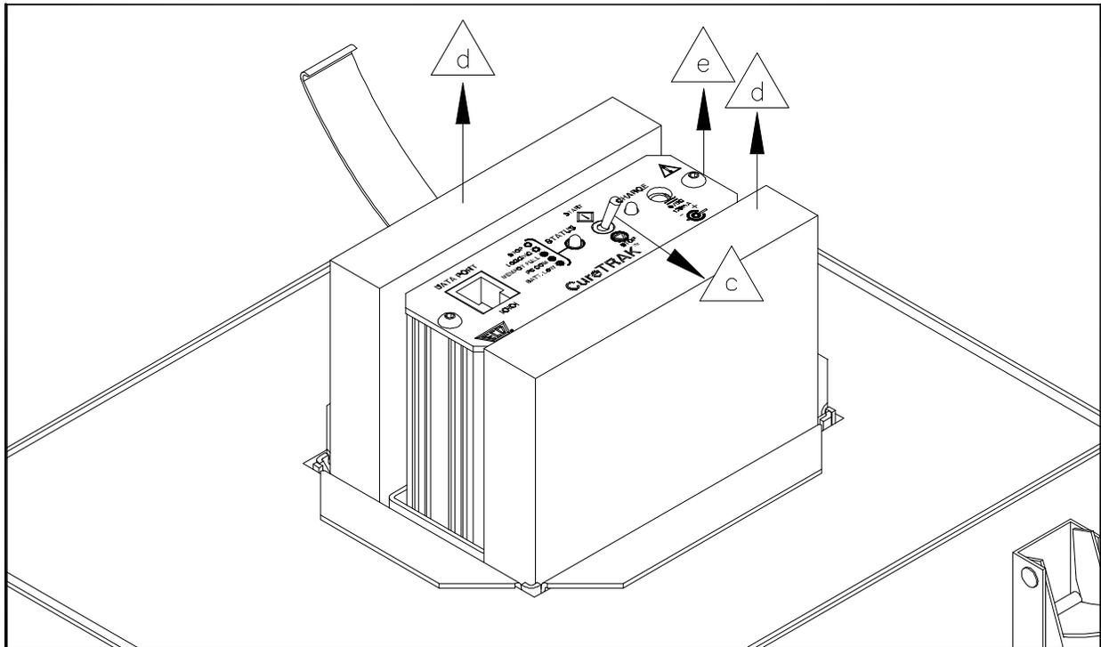
**Figure 4-9: Data Box Removal**
