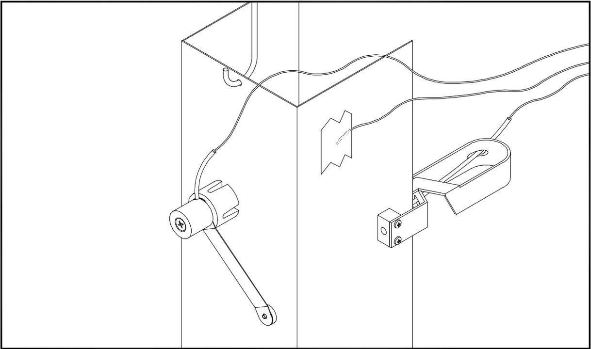
*Figure 4-8: Sensor Attachment*
