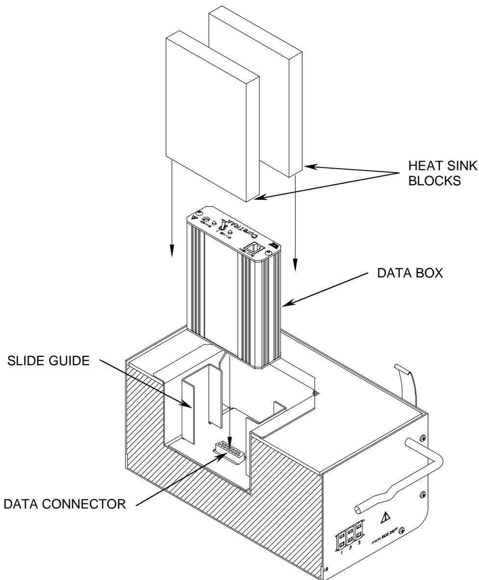
**Figure 2-3: Thermal Barrier Interior Features**
