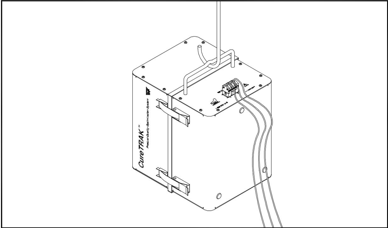
*Figure 4-7: Hanging the Thermal Barrier*
