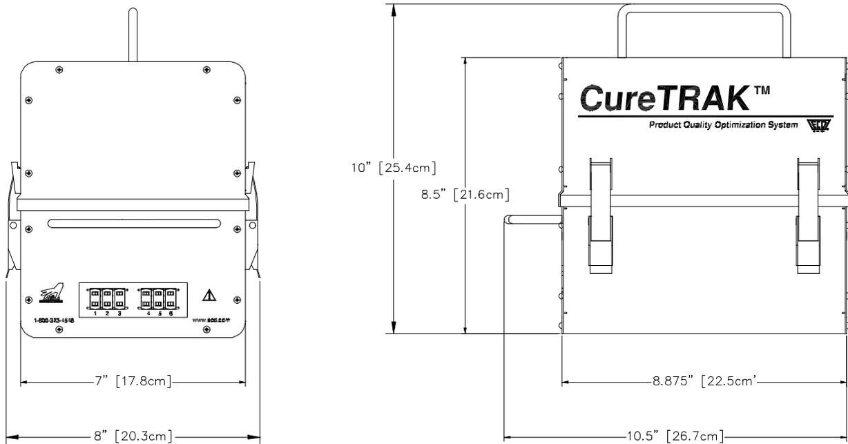
**Figure A-1: Thermal Barrier Exterior Dimensions**
