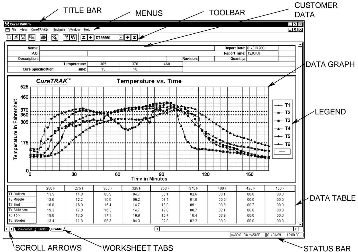
Figure 2-5: Cure Conformance Software
