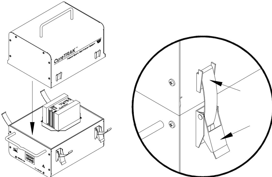
**Figure 4-5: Securing the Barrier Top**
