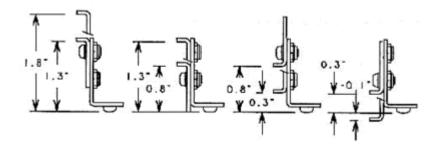
Figure 1: Rail Adjustment Range
