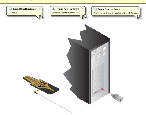
The Transceiver can either be connected directly to a computer USB Port or a USB extension cable. Using an USB extension cable can be a simple way to get the Transceiver to a better reception area without moving the PC. No matter which method is used, keep wires and other metal objects away from the Transceiver.
