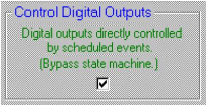
When this option is selected, the digital output names must match the event names as described in *Defining Inputs and Outputs* earlier in this chapter. The outputs must be named as described in *Assigning Input/Output Names* in the next section, and at least one state with one exit condition must be defined, even if you are not using the Mode\_Out output from the State Machine functional block.
