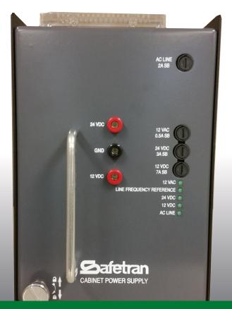
▷ ▷ The PS-250 unit, which supplies regulated DC power, unregulated AC power, and a line frequency reference for the Detector Rack, BIUs, load switches, and other auxiliary equipment.
