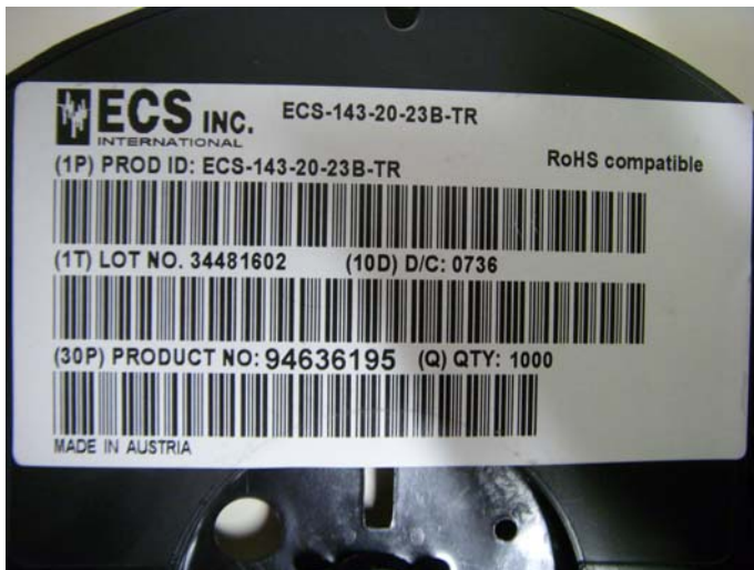
Photo 1) Label of counterfeit product. Not ECS format.
