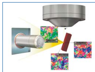
Figure 2 – Schematic of EBSD detector, sample and electron beam geometries in SEM chamber.
