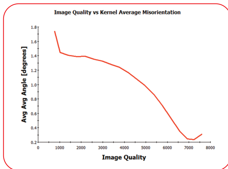
Figure 3. Correlation plot of Image Quality vs. Kernel Average Misorientation (KAM) for a dual phase steel microstructure. This plot indicates that in general, as pattern quality improves the local misorientation decreases, as expected for a ferrite-martensite structure.
