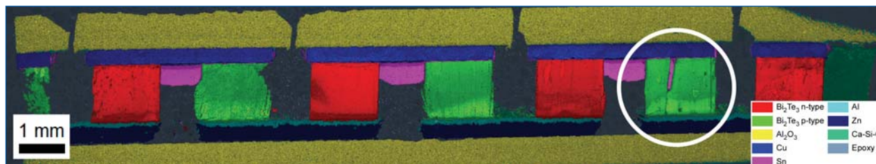
Figure 2: Phase map derived from simultaneously collected EBSD and EDS data with highlighted defect.
