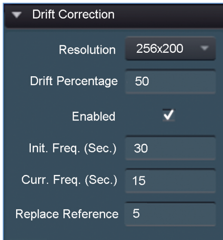
Figure 3. Drift Correction software panel and parameters used during an analysis. In this case the initial drift correction images were collected every 30 seconds. However, after collected images demonstrated that there was drift, the frequency of collection was automatically changed to 15 seconds.
