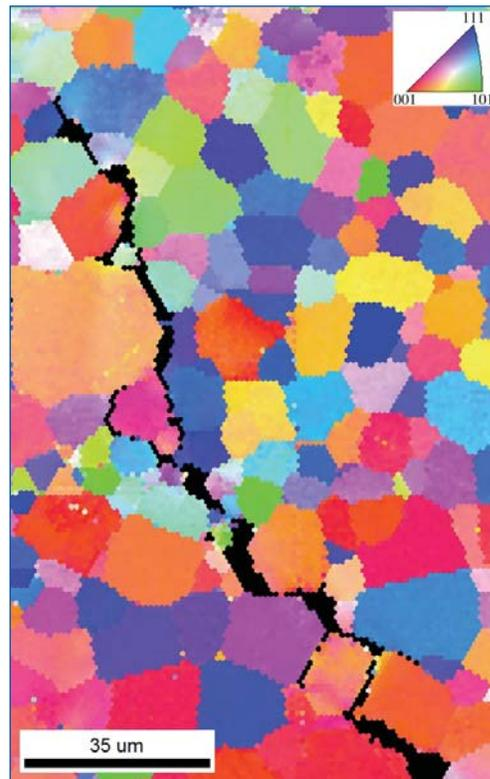
Figure 2 – An inverse pole figure map showing the EBSD data obtained from OIM around a stress corrosion crack found in the corroded 2124 aluminum alloy.
