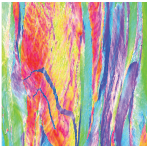
90µm Figure 1: Deformed Copper – An Orientation map from a 75% cold rolled high purity copper sample. The large amount of deformation present produces significant orientation changes within parent grains. OIM can be used to investigate the correlation of orientation to deformation behavior.
