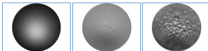
Figure 4 – Difference between standard background subtraction and enhanced processing on an oxidized magnesium alloy specimen. Left: EBSD pattern as detected, middle: pattern after standard background subtraction, right: pattern after enhanced processing using the recipe given above. The enhanced processing allows successful scanning of the sample.
