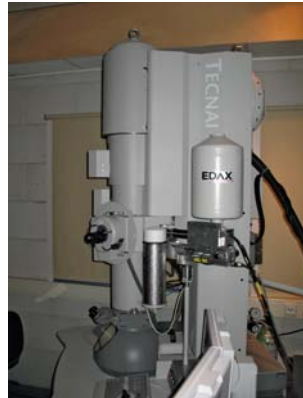
FEI Tecnai G 2 F20 XTWIN with EDAX r-TEM detector.
