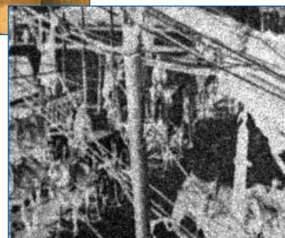
Figure 2b: Ag(L) element image of photo using 30 \mu\text{m} poly-capillary at 250 DPI pixel density.
