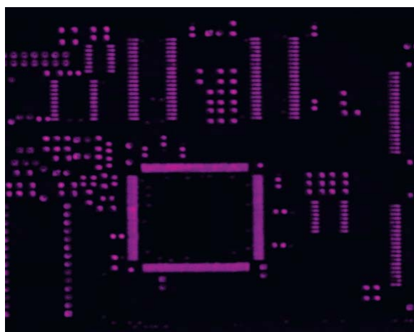
Figure 4: Orbis Pb(L) elemental map of a PCB using a 1 μm collimator. The map indicates the use of Pb-based solder to mount the components on the board.
