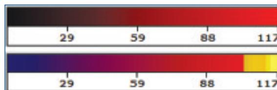
Figure 2b: User palette (above) shows grayscale for Ti(K). The custom user palette (below) employs ramped colors on the low intensity end of the palette. A few of the indices on the high intensity end have been manually altered to high-light hot spots in the map.
