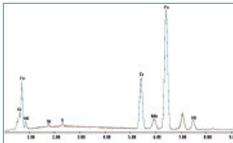
Overlay of stainless steel spectra collected at 5K, 10K, 20K, 40K, 60K, 80K, and 100K, by Apollo XV SDD.
