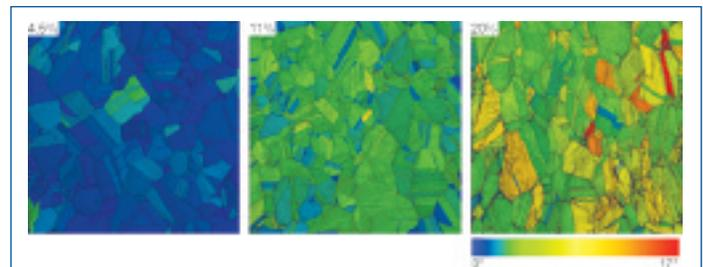
Figure 4: Combined Image Quality and Grain Orientation Spread maps.
