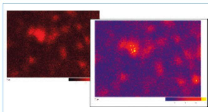
Figure 2a: Ti(K) XRF map shown in grayscale and also shown with a user palette containing areas of high concentration in yellow.
