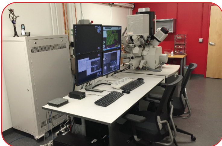
Figure 1. University of Arizona Lunar and Planetary Laboratory with an FEI Helios dual-beam FIB-SEM and EDAX TEAM™ Pegasus Analysis System.
