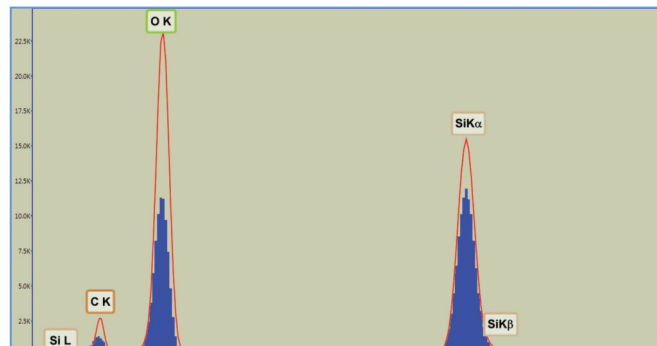
Spectra of SiO 2 collected with the Octane T Plus detector (red) compared to a SiLi Detector (blue) have been normalized to the highest energy part of the spectrum. The Octane T Plus detector significantly improves the low energy sensitivity. The Si K intensity is improved by 30% and the O K by 150%
