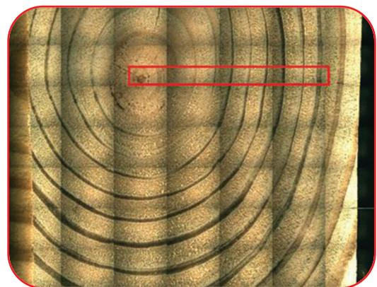
Figure 2. Montage image of wood cross-section sample, with mapping area highlighted in red. The wood sample has been treated with a copper micro-particle preservative.
