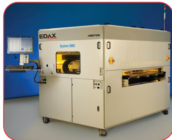
Figure 1. XLNCE SMX-ILH XRF Analyzer.
