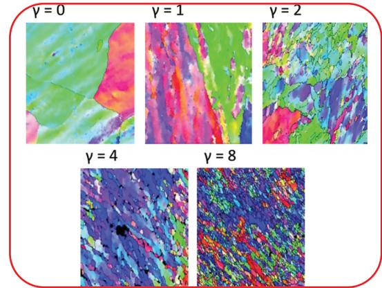
Figure 2. Microstructure of Al after different shear strains processed by ECAP.
