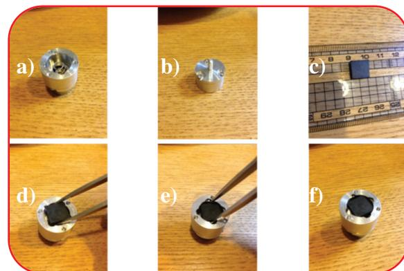
Figure 1. The holder created by Takashi. (a) Top, (b) bottom, (c) the sample, (d) placing the sample in the holder, (e) rotating the sample into place, and (f) the finished mounted sample.
