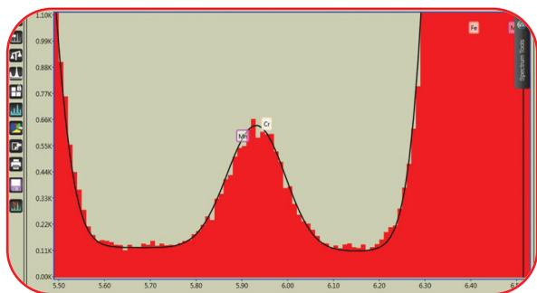
Figure 2. Same steel sample with  $\text{CrK}\beta$  and  $\text{MnK}\alpha$  (overlapping) identified (perfect HPD fit).
