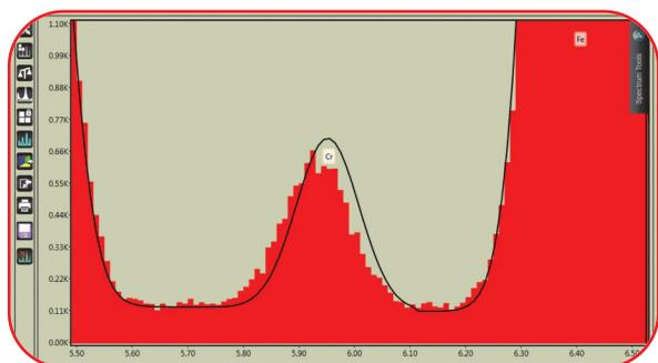
Figure 1. A steel sample with only Cr identified (HPD misfit).
