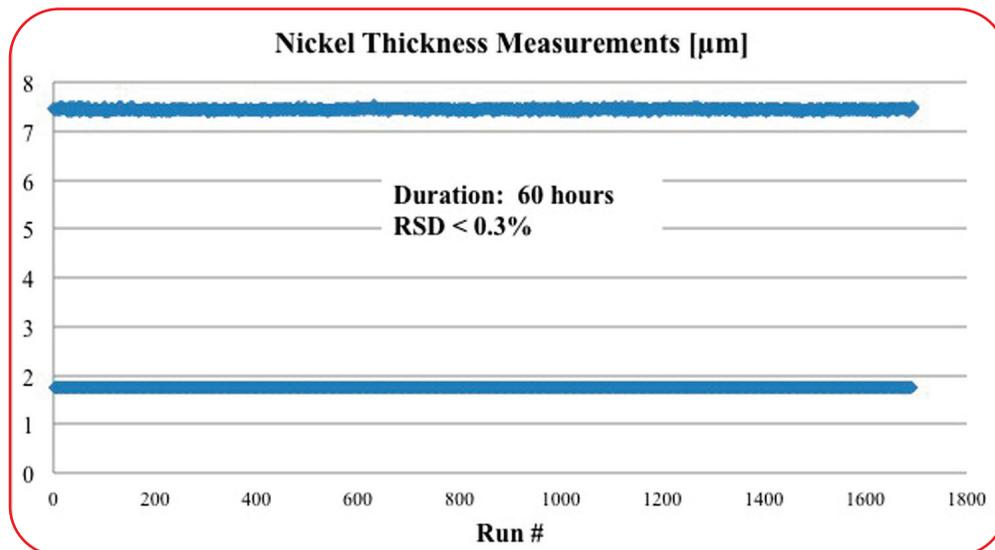
Figure 2. Measurements of two different Ni plating thicknesses using the SMX-ILH over the course of 60 hours. The plot shows precision better than 0.3% RSD.
