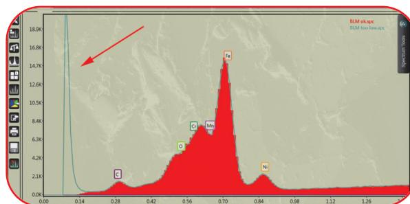
Figure 4. BLM set incorrectly (cyan) and set correctly (red).
