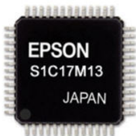
16-bit S1C17M13 MCU with integrated Flash Memory
