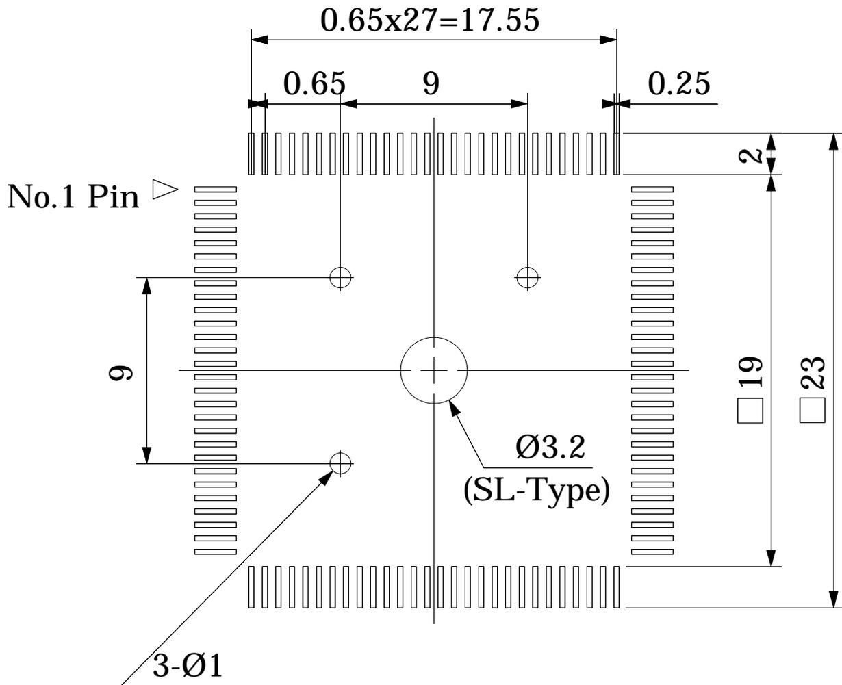
\* Recommended foot pattern shown on left is for NQPACK soldering.
