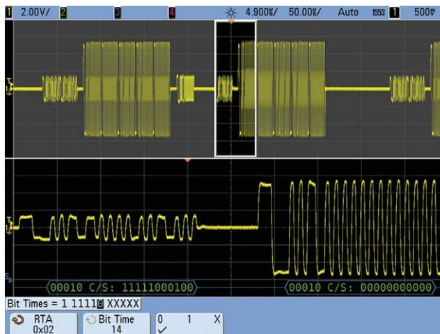
**Figure 8. Setting up the scope to trigger on a specific Command Word with the transmit bit set.**
