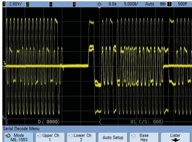
Figure 3. Initial MIL-STD 1553 decode and trigger setup using “Auto Setup”.
