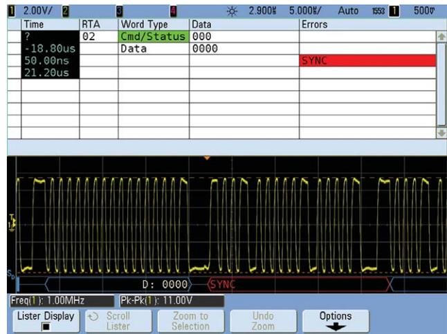
Figure 10. Triggering on a “Sync” error condition
