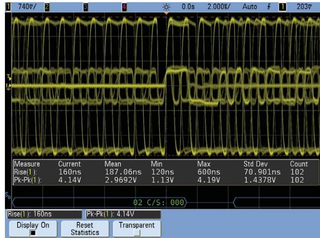
**Figure 6. Conventional oscilloscope edge triggering fails to isolate specific input/output Words and messages for analog parametric characterization**
