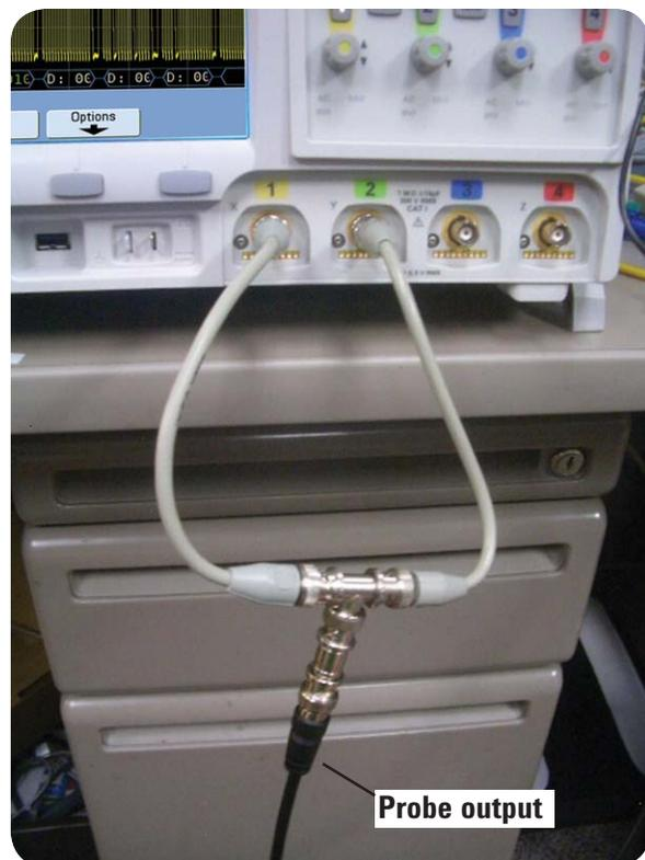
**Figure 2. Connecting the N2791A differential active probe to two channels of the oscilloscope.**
