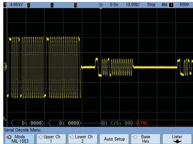
**Figure 4. Insufficient signal swing produces erroneous "Sync" error.**
