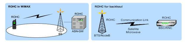
WiMAX Forum Network Architecture Release 1.5 – Stage 3 for Detailed Protocols and Procedures Base specification for ROHC support describes the system architecture and signaling procedure for ROHC. It supports the following ROHC framework and profiles implemented in the form of various Effnet products:
