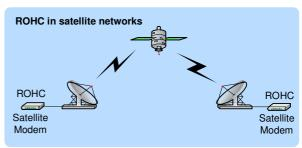
Effnet ROHC-TCP<sup>TM</sup> provides improved bandwidth efficiency when used together with Protocol Enhancement Proxies on satellite networks, bandwidth optimization techniques in WAN optimizers, TCP accelerators and on backhaul links.
