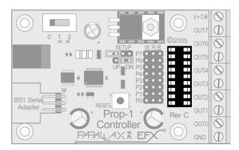
**Permanent Installation**: When the Prop-1 Trainer is to be integrated into the prop control circuitry, the best thing to do is remove the ULN2803 and replace it with the ULN2003. The ULN2003 has seven circuits and can be aligned such that it does not interfere with POT circuitry on P7. Correct alignment of the ULN2003 is shown below – note that the top two pins of the ULN2803 socket are not used.
