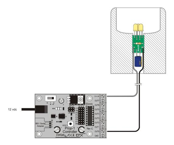
Note that the Prop-1 power switch must be set to position 2 for the WickLED(s) to operate. When more than three WickLEDs are connected to the Prop-1, you may want to connect a single common wire (#16, stranded) to the V+ terminal and use a wire-nut to connect the WickLED common (striped) wires to it.
