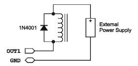
Note the addition of the 1N4001 suppression diode when using the external supply. This is recommended because the diodes internal to the ULN2803 are not connected to the external supply when using this configuration.
