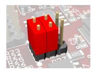
JP2 The RS-485 interface is half duplex. Only two wires are needed for communication, but an additional port bit is required to switch between receive and transmit mode. Thus pins 1 and 2 as well as pins 3 and 4 of JP2 must be shortened to control the data direction via ATmega port bit PD5.
