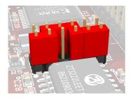
JP1 Hardware Handshake can also be used, if UART1 is routed to the RS-232 interface.
