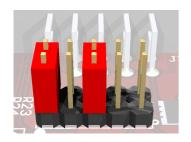
JP5 Jumper JP5 routes the JTAG signals to the ATmega128, if pins 1 and 2 and pins 5 and 6 are shortened.
