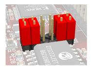
JP1 Most applications will probably use UARTO for RS-232 and UART1 for RS-485. This configuration is shown here. Pins 1 and 2, 3 and 4, 9 and 10 and 11 and 12 of JP1 are shortened.
