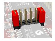
JP1 Shortening pins 1 and 2 and pins 11 and 12 will route UARTO transmit and receive lines to the DB-9 connector.
