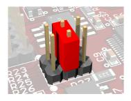
JP2 The direction signal is pulled low by R27. If pins 3 and 4 are shortened only, the RS-485 interface is configured as a receiver and no port bit for direction control is required.
