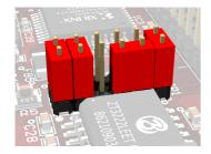
JP1 Even both UARTs can be routed to the DB-9 connector when shortening pins 1 and 2, 3 and 4, 7 and 9 and 11 and 12. However, a special adapter is required to route the UART1 transmit line from the on board DB-9 pin 7 to a second DB-9 pin 3 and the receive line from the on board DB-9 pin 8 to pin 2 of the second connector.
