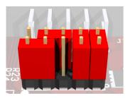
JP5 Routing the JTAG interface to the CPLD is provided by shortening pins 1 and 3, 4 and 6, 7 and 8 as well as pins 9 and 10. However, you need a special Xilinx adapter for programming the CPLD via JTAG.
