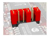
JP1 If your application requires hardware handshake via RTS/CTS, then connect JP1 pins 4 and 6 and pins 5 and 7. The picture on the right shows the hardware handshake configuration for UARTO.
