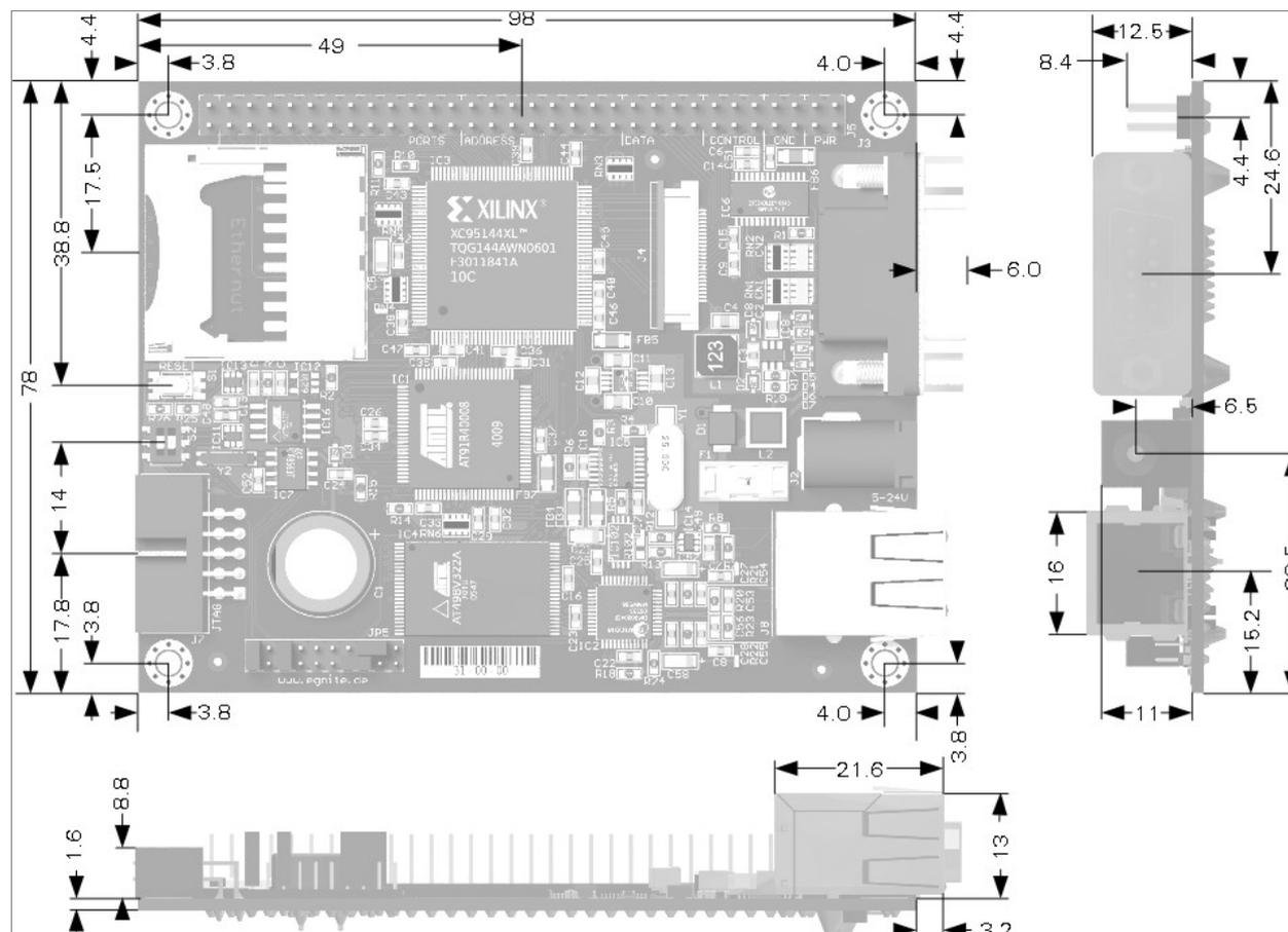
Ethernut has four 3mm mounting holes. Except for the mounting hole close to the Ethernet connector, all remaining holes are internally connected to the Ethernet, RS-232 and MMC socket shield. Conductive mounting bolts may be used in these positions to provide a good connection to a metal housing. This will minimize electrical and magnetic radiation.
