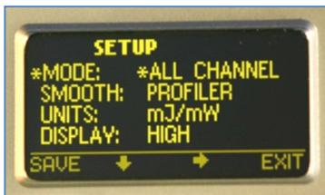
For the best match between PowerView II and the instrument display, select SMOOTH: PROFILER in SETUP Mode.
