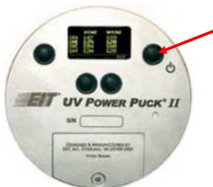
Depress the Power button to energize the radiometer
