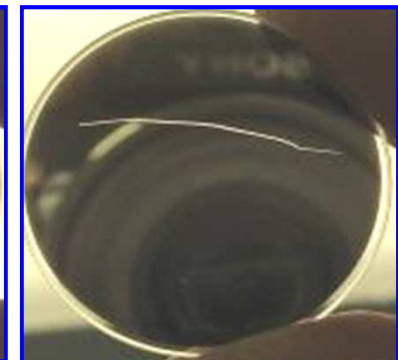
Customer Returns: Left: Improper Cleaning Right: Scratch
