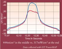
Figure 9: Comparison of measurements at the end of the bulb, versus near the middle. If the readings are lower in the middle than on the end, opposite of what is shown here, check the positioning of the bulb and look for sag.
