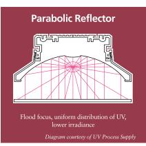
Figure 6: Typical light pattern from a Parabolic Reflector design.
