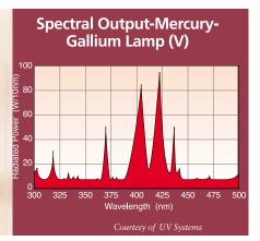
Figure 19: Typical Spectral output from a Mercury Gallium Lamp (Courtesy of UV Systems).
