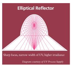
Figure 5: Typical light pattern from an Elliptical Reflector design.
