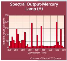
Figure 17: Typical Spectral output from a Mercury Lamp (Courtesy of Fusion UV Systems).
