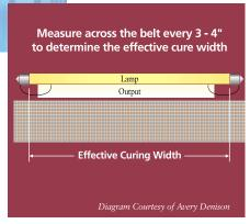
Figure 11: Procedure to find the effective cure width with your radiometer (Courtesy of Avery Dennison).
