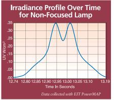
Figure 8: Typical light pattern from lamp that is out of focus. It is important to confirm if your process and equipment was designed to run out of focus or if the out of focus condition is a change due to a bulb sagging or lack of maintenance.
