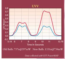
Figure 16: Looking at only the UVA, the old and new bulbs appear to be similar in output. There is quite a difference in the output of UVV with the new bulb significantly. It is important to sometimes measure more than a single UV bandwidth. (Information originally collected by Efsen Engineering).
