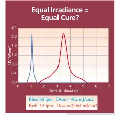
Figure 21: Equal numbers of Watts do not always lead to equal cure characteristics. It is important to establish and maintain energy density levels for your process.
