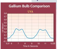
Old Bulb: 537mJ/309mW New Bulb: 487mJ/290mW
