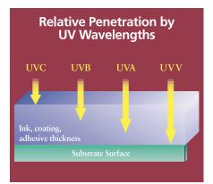
Figure 15: The longer wavelengths have a better chance for penetrating through coatings than the shorter wavelengths.
