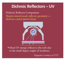
Figure 13: UV energy is reflected to the substrate while the amount of IR is minimized (Courtesy of UV Technology).
