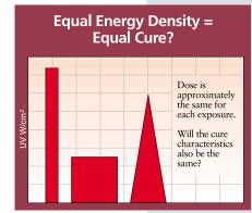
Figure 22: Equal numbers of Joules do not always lead to equal cure characteristics. It is important to establish and maintain irradiance levels for your process.
