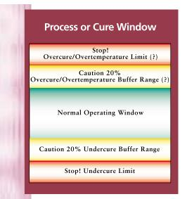
Figure 23: An easy to understand graphic of the Process or Cure Window. Establish the window for your process and stay in the green zone. A radiometer can report the highest irradiance measured (peak irradiance) and/or a profile of the irradiance over time (irradiance profile).
