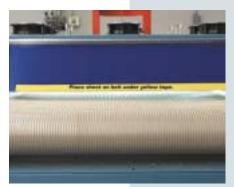
Figure 10: Yellow tape attached to the UV system to guide product placement on the UV conveyor (Photo courtesy of Avery Dennison).
