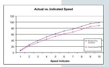
Figure 2: Small variations in the actual versus the indicated process speed are expected. Confirm and document your dwell time independently.
