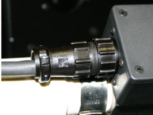
**Figure 8**-Close-up of connector on Heater Assembly. This connection has been made at the factory prior to shipping and should not be disconnected
