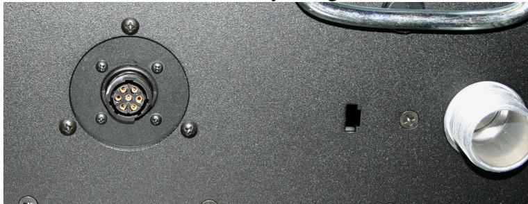
**Figure 4-(Above) Heater Power/Sensing connection on left, hose connection on right**
