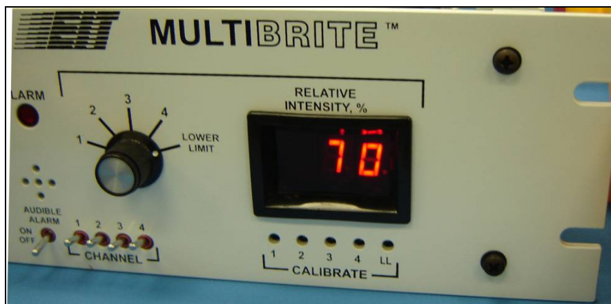
Figure 58: Low Level Threshold
