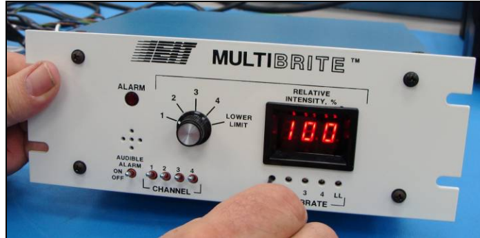
Figure 57: Channel 1 100% Baseline Calibrate POT
