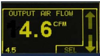
Display shown in Flow Rate Mode (4.6 CFM)
