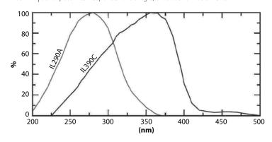
**FIGURE 5** | Band-pass filter response for a four-channel radiometer.
