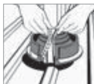
2. Place the Dektite® around the pipe and engage metal teeth in opposing pockets starting at the top.
