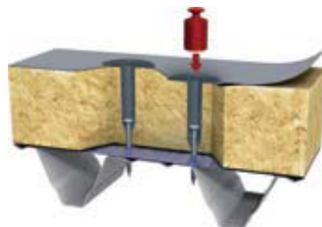
Telescope design for resistance to imposed loads
