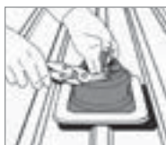
1. Adjust Dektite® to the pipe.
