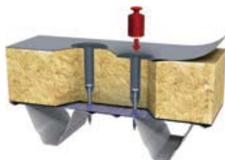
Telescope design for resistance to imposed loads
