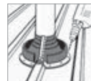
5. Fasten Dektite® with EJOT® self-drilling screws or bulbrite rivets.
