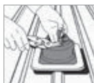
1. Adjust Dektite® to the pipe.
