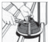
1. Adjust Dektite® to the pipe.
