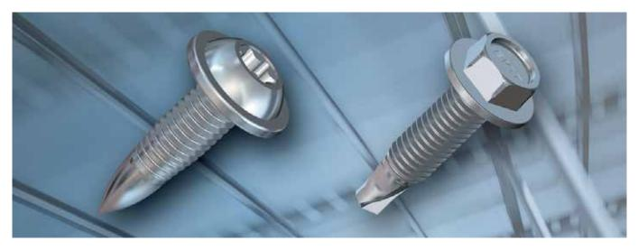
The <u>EJOT FDS</u><sup>®</sup> flow drilling screw enables a high strength screw joint, due to increased thread engagement in the formed draught.
