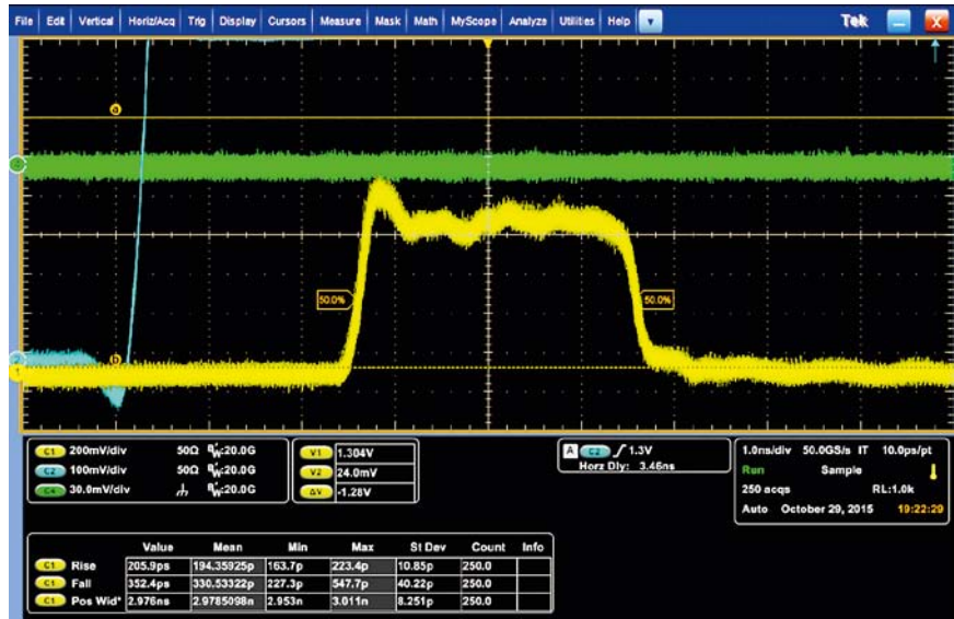
Fig 2. Example of temporal pulse shape, stability of pulse shape
