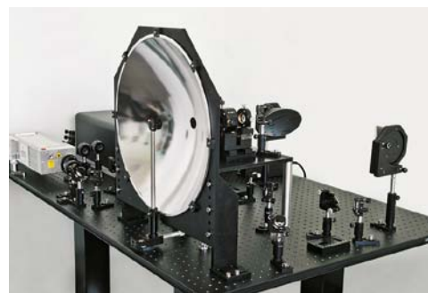
Fig. 3. T-SPEC THz spectrometer installed into LIDAR operating in terahertz range was used to scan remote objects at 7 m distance.
