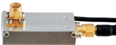
Fig. 6. External view of preamplifier
