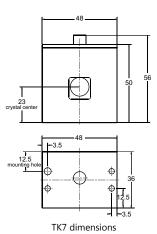
TK7 is compact oven with build-in thermocontroller for temperature up to 60 °C. TK7 oven provides more crystal mounting options in comparison to TK3 or TK4. Like in KK1, each crystal is mounted into adapter before insertion in oven. TK7 and KK1 crystal adapters are compatible. Maximum crystal size for this model is 12×12 mm and the length of the crystal – 30 mm.
