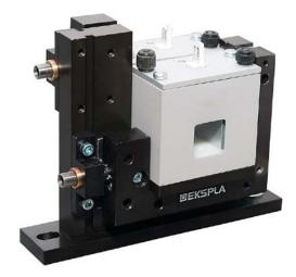
**H2 type mount** can fit two TK3, TK4 or TK7 type ovens and is ideal for holding second and third or fourth harmonics generators.
