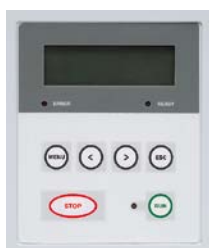
Fig. 2. Front panel controls of PS5050 flashlamp driver
