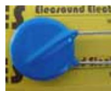
Varistor is a voltage dependent resistor. Which have symmetrical voltage-current characteristics and unparalleled large peak current capability are used for absorption of transient voltage, suppression of pulse noise and circuit voltage stabilization.
