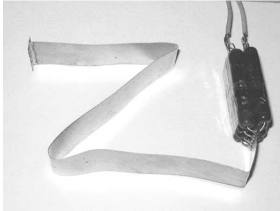
Figure 4.35 Setup showing the dc resistance measurement.
