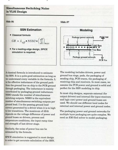
Figure 3: Page 5 of Liren Chen's paper showing the simultaneous switching noise estimation and circuit model.
