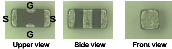
Figure3.Feed Thru Capacitor (0603 case size with 1uF,BJ)
