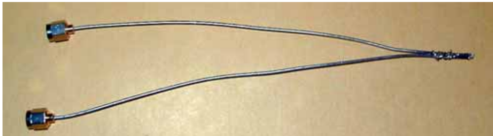
Figure 9: Low inductance wire fixture used to measure MLC capacitors.
