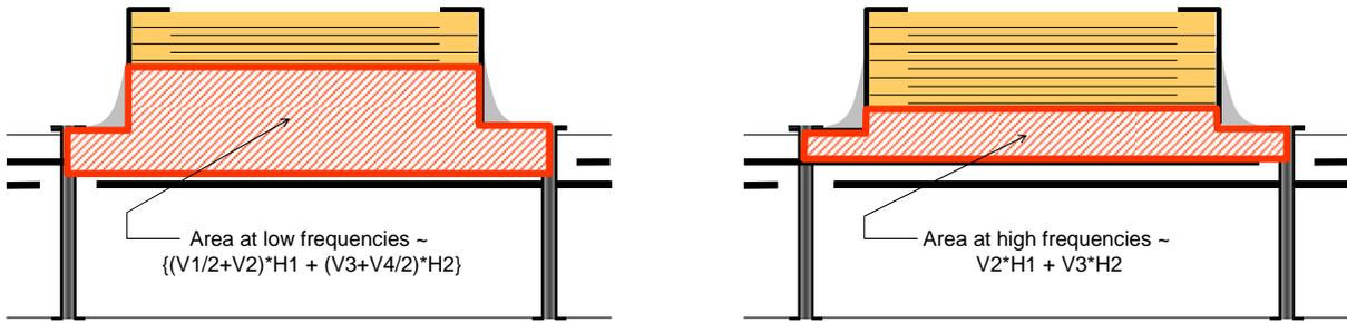
Figure 3. Illustration of approximate current-loop shapes and cross-section areas. On the left: low-frequency model; on the right; high-frequency model.
