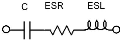
Figure 1. Simple RLC equivalent circuit of a capacitor.
