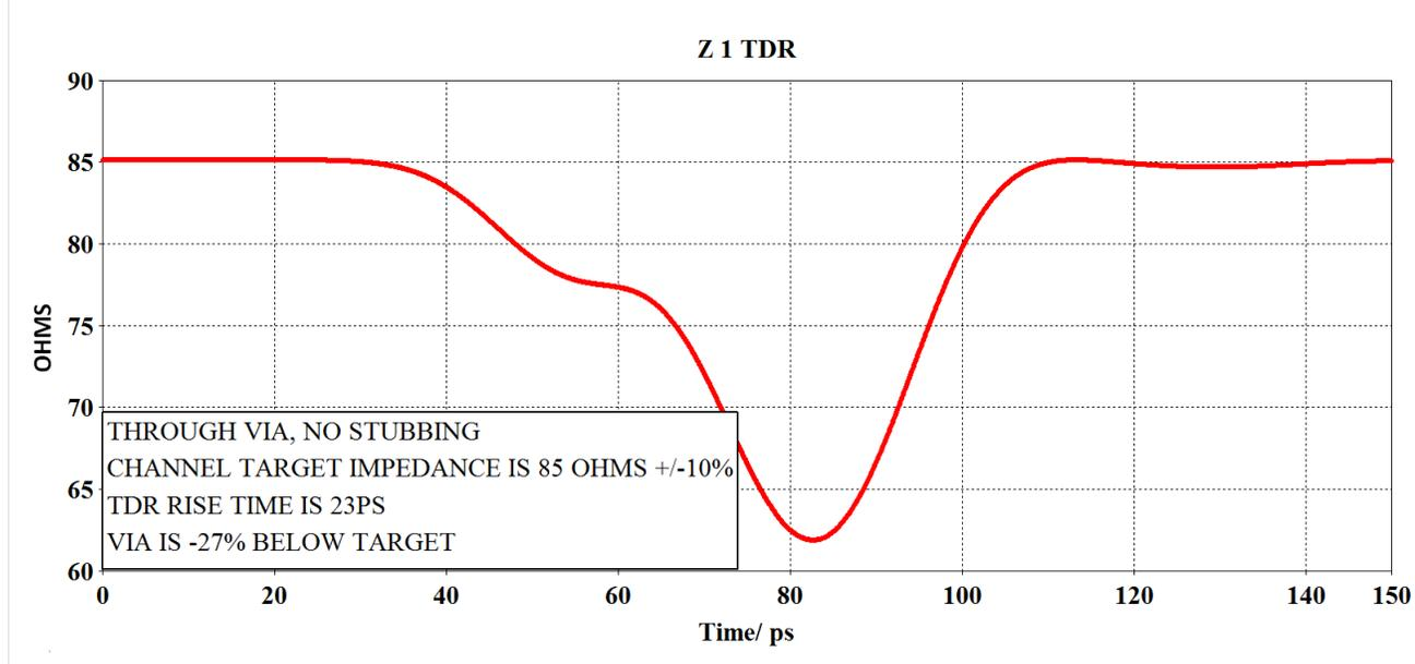
*Figure 6* Through via showing impedance discontinuity
