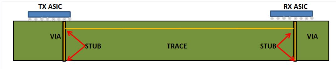
Figure 3 Example of via stubbing
