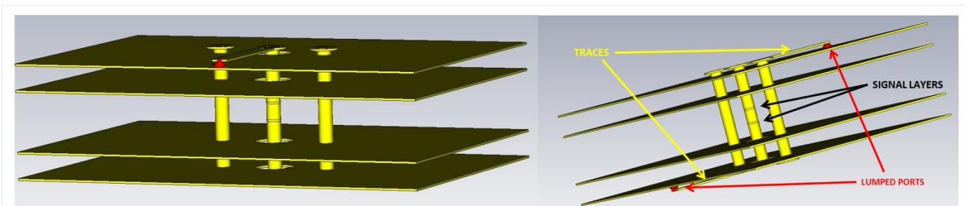
Figure 9 Simple 8 layer PCB stack
