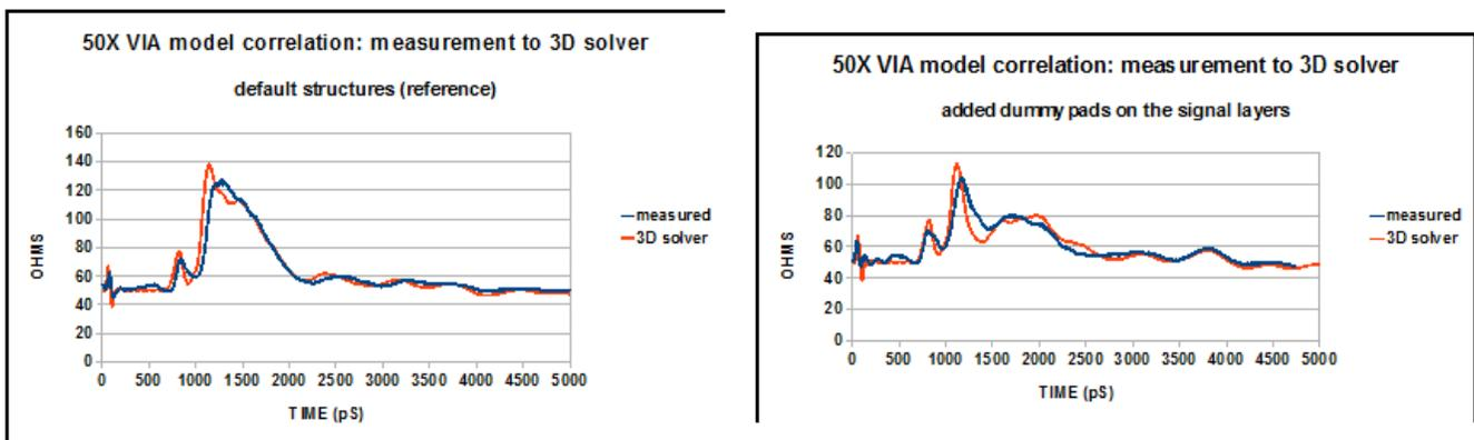
Figure 31 50X scaled model measured and simulated: default vs added signal pads
