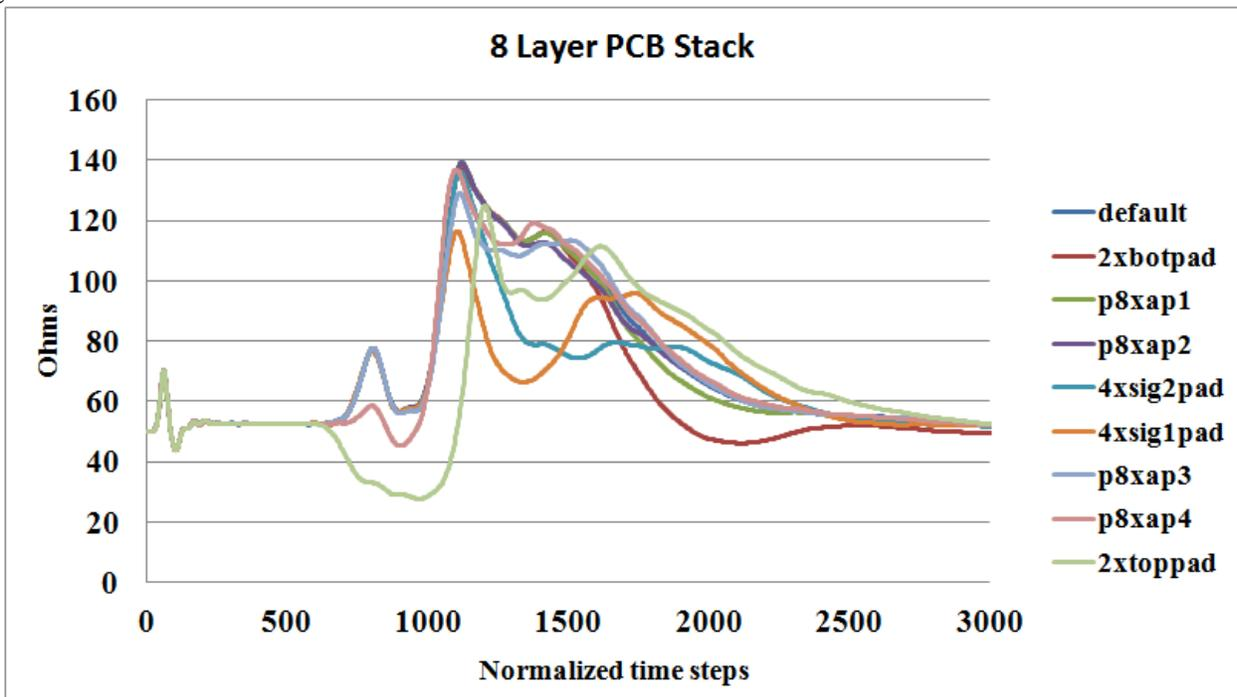
Figure 16 8 layer PCB sub-structure responses with a 2ps rise time TDR
