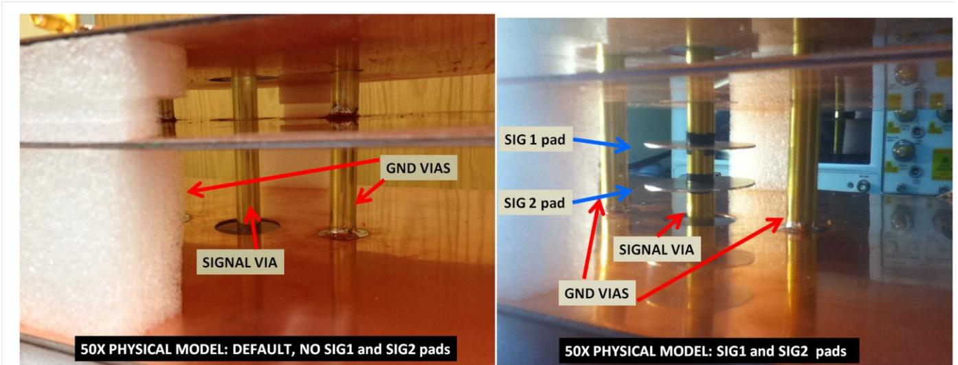
Figure 30 Details of the 50X physical model
