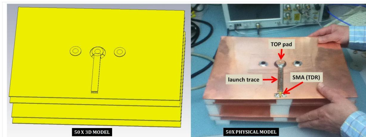
Figure 19 50X 3D model versus 50X physical model
