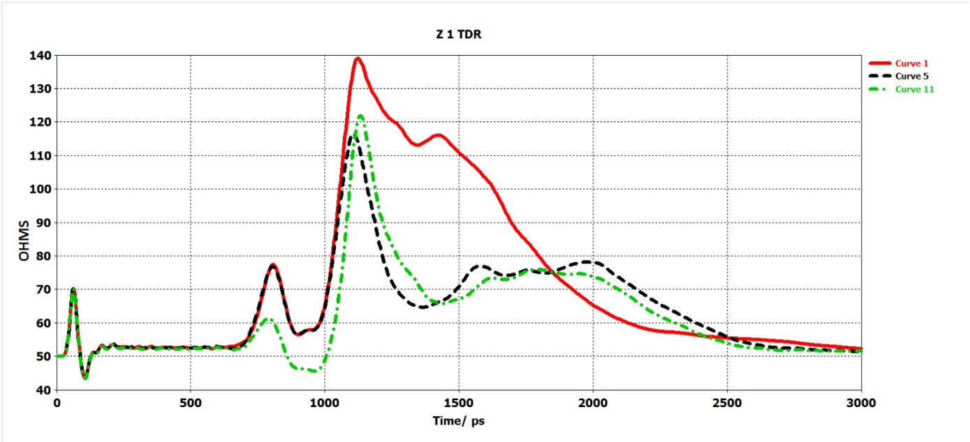
Figure 25 Final optimization, top and bottom pad diameters increased, TDR rise time=30ps
