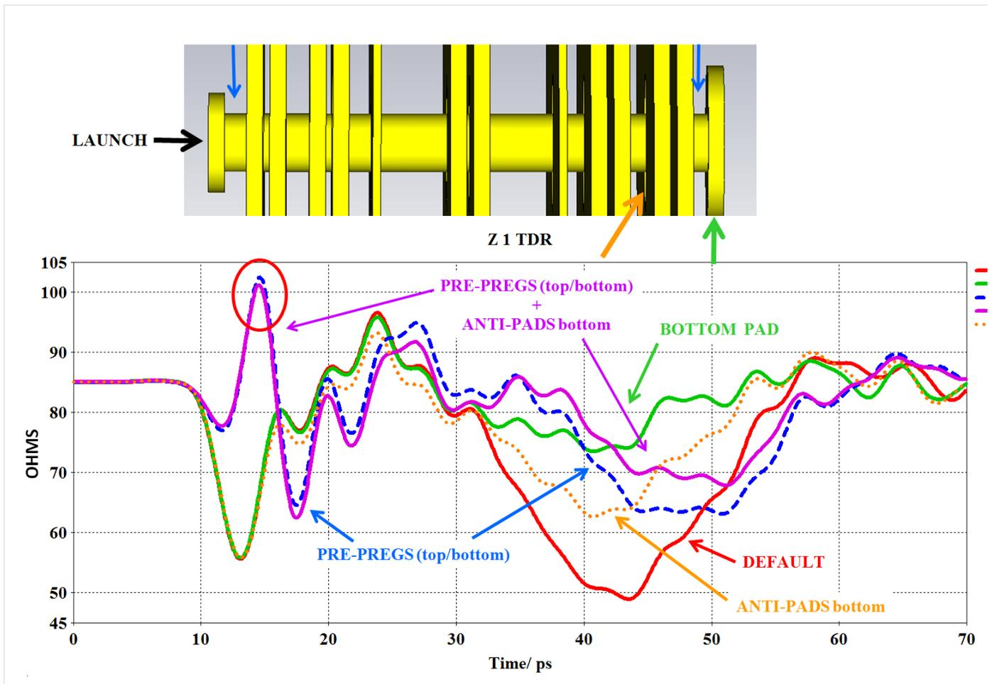
*Figure 13* 16 layer PCB stack, default structures vs bottom pad reduction, TDR rise time=2ps
