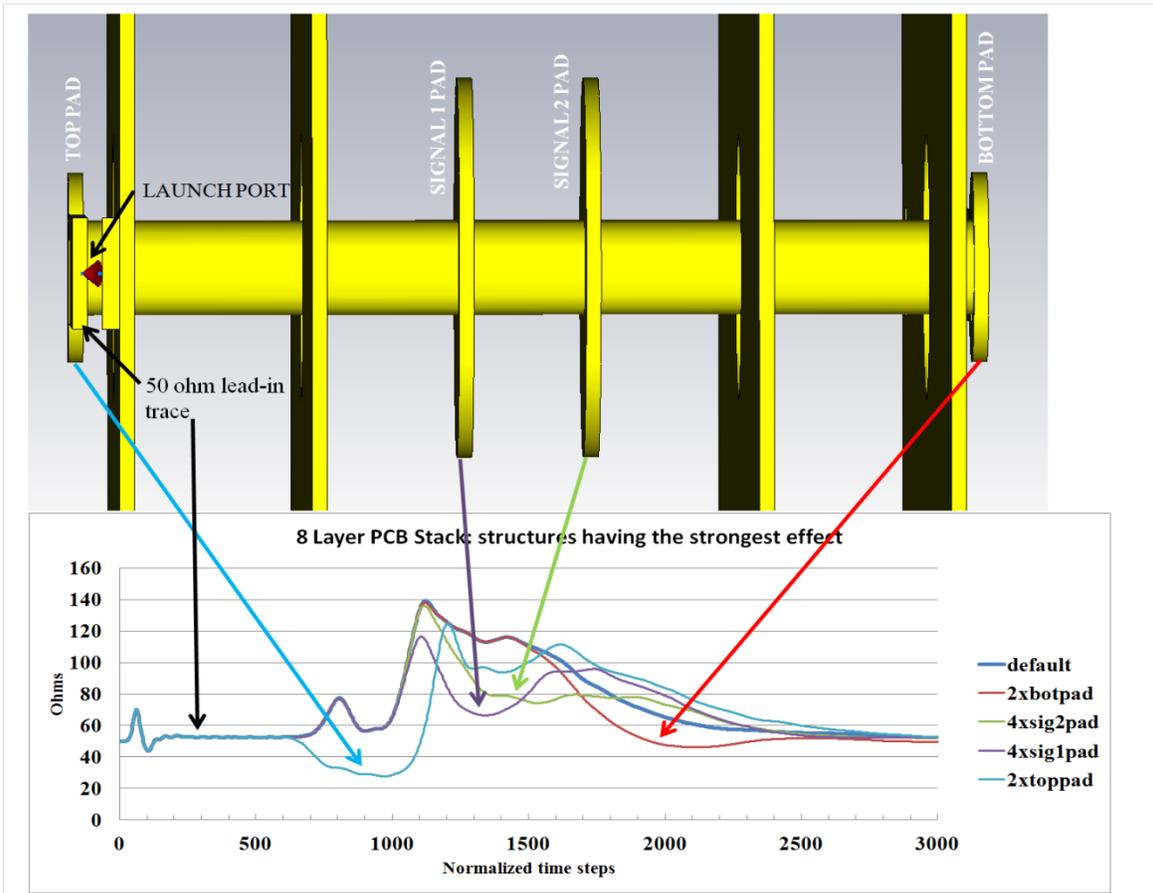
*Figure 17* 8 layer PCB stack, 2ps TDR responses: sub-structures with strongest effect on impedance
