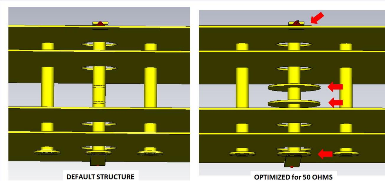
Figure 26 Comparing metal sub-structure changes for 50 ohm optimization
