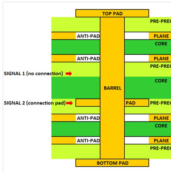
*Figure 1 Basic through via cross section and detailed anatomy*
