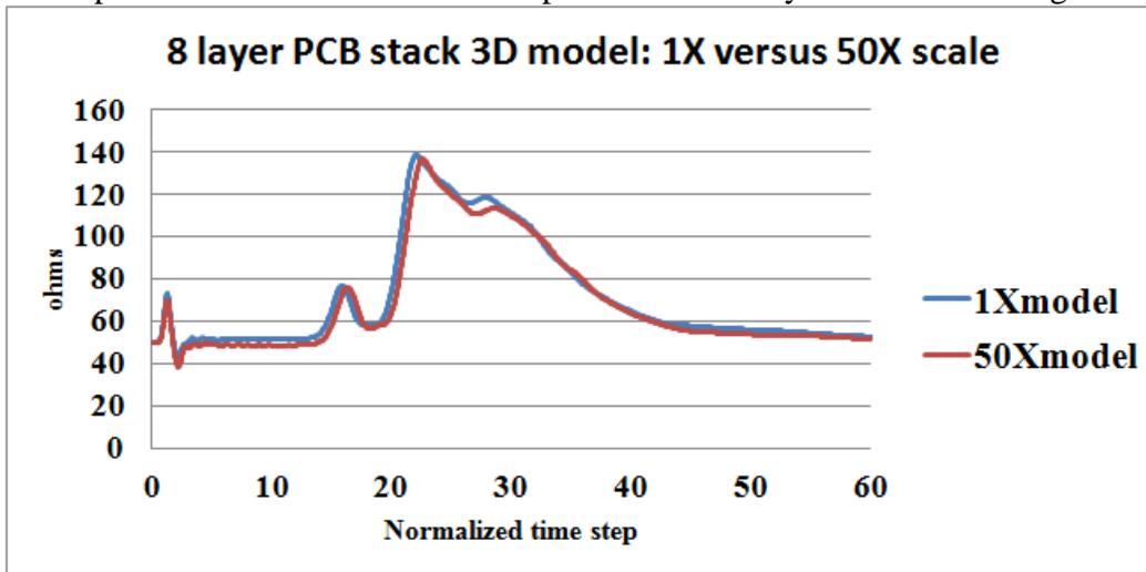
*Figure 20 8 layer PCB stack 3D model comparison: TDR 1X vs 50X*
