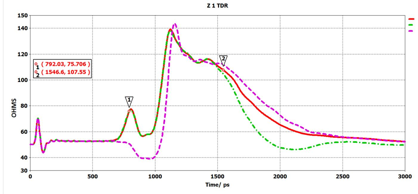
Figure 21 End to end structure time calibration, TDR rise time=30ps
