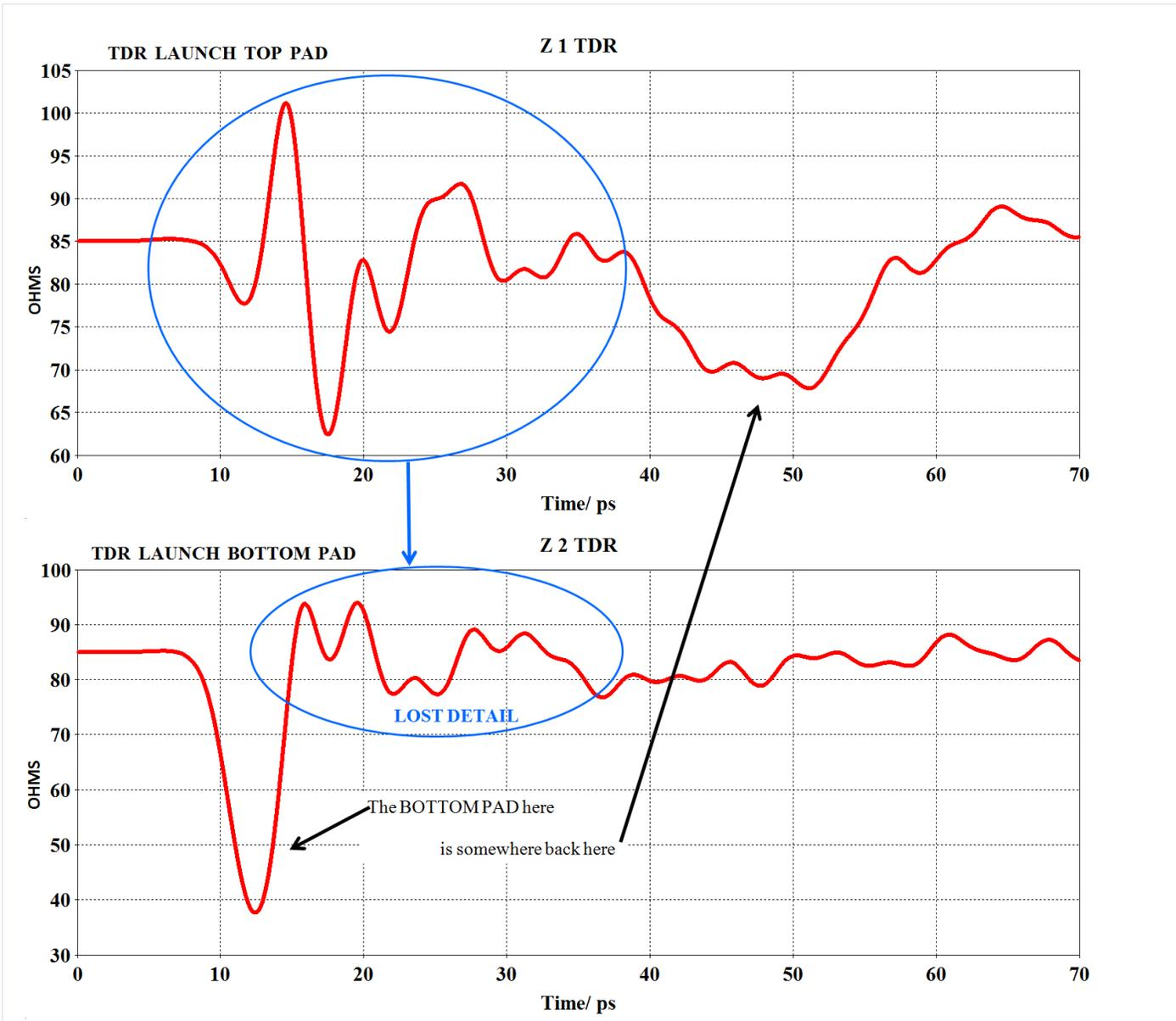
Figure 14 16 layer PCB stack contrasting launch Top pad vs Bottom pad, TDR rise time=2ps
