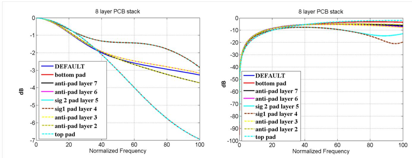
Figure 10 8 layer PCB stack insertion loss responses
