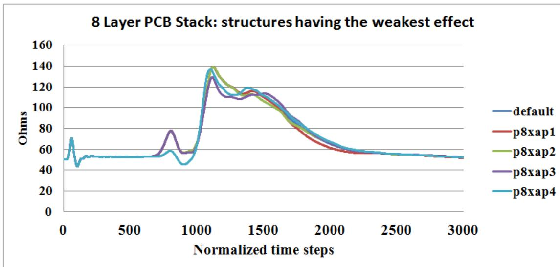
*Figure 18* 8 layer PCB stack 2ps TDR responses: sub-structures with weakest impact on impedance
