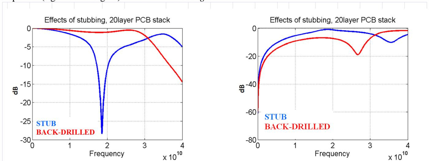
Figure 5 Effects of stubbing on insertion and return loss
