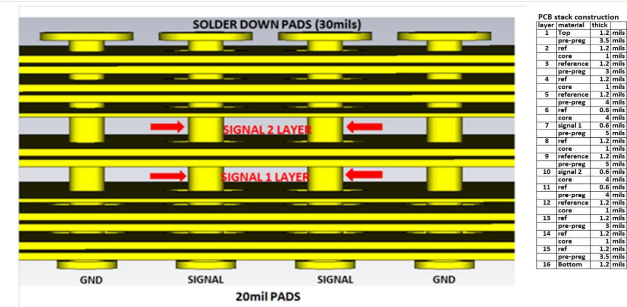
Figure 7 16 layer dense stack with special pad requirements
