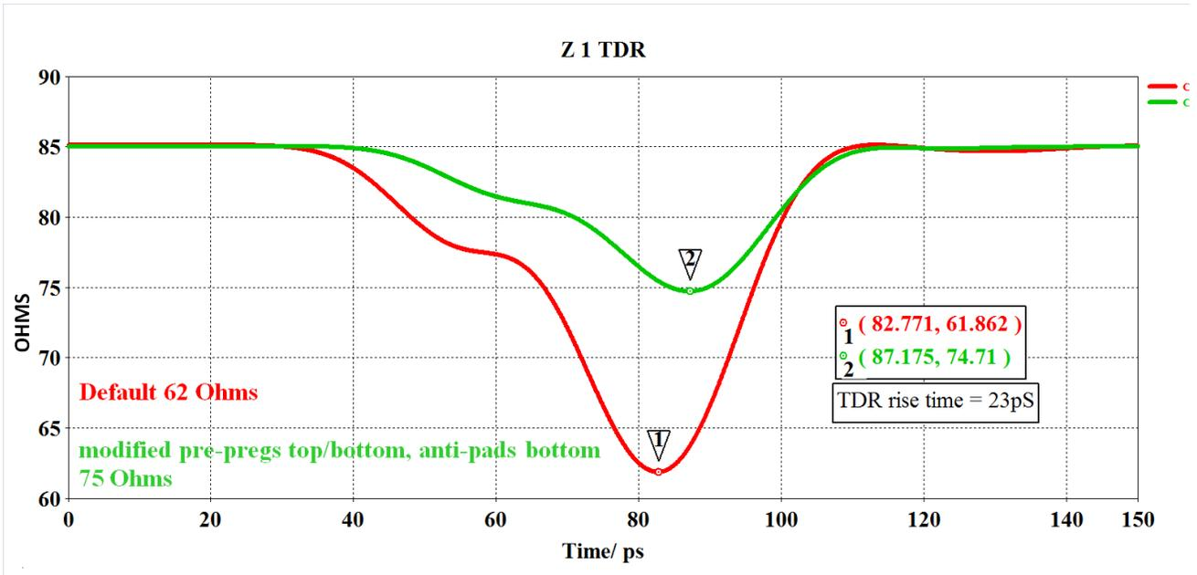
*Figure 11* 16 layer PCB stack, default structures vs adjusted anti-pads and top/bottom pre-pregs , 23ps TDR
