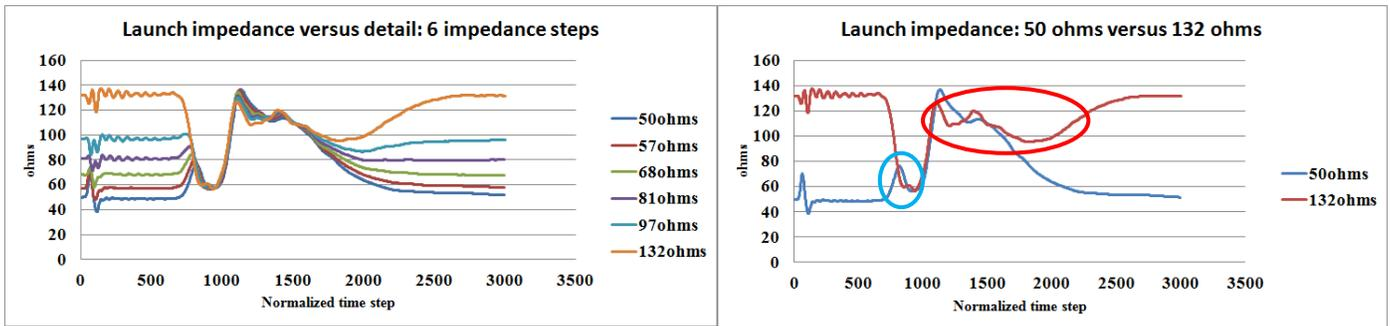
Figure 15 8 layer PCB stack, launch impedance vs trace detail
