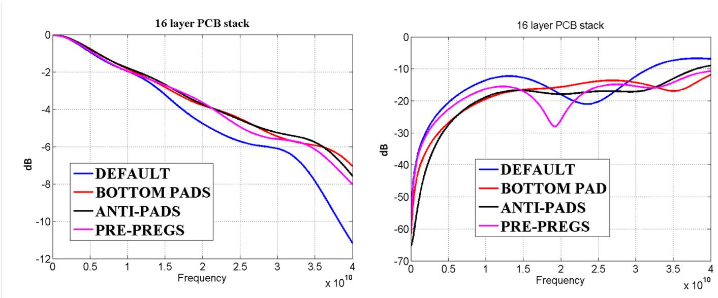
Figure 8 16 layer PCB stack insertion and return loss responses
