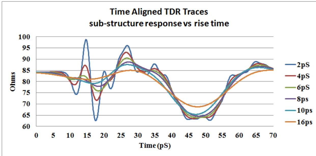
*Figure 12* 16 layer PCB stack, TDR rise time response
