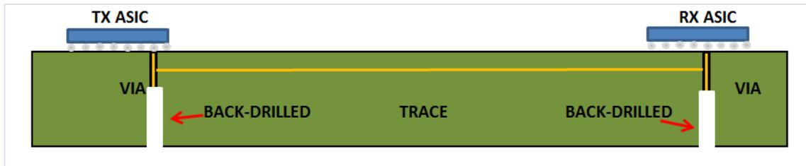
Figure 4 Example of back-drilled vias
