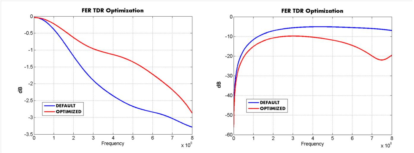
Figure 27 FER TDR optimization, insertion (left) and return loss (right) plots
