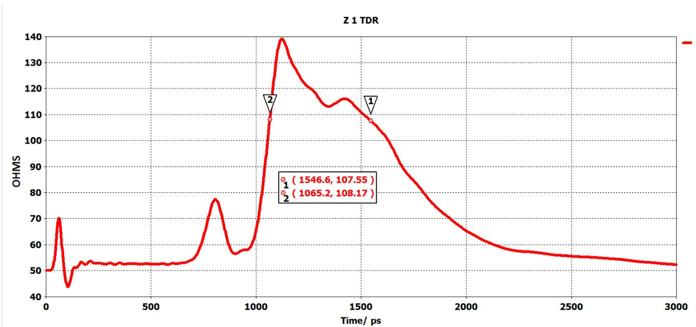
*Figure 22* First impedance discontinuity target, TDR rise time=30ps
