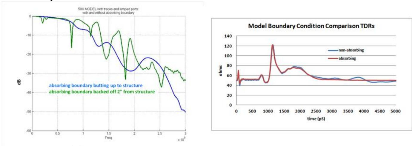
**Figure 29** Contrasting boundary conditions Frequency domain (left), Time domain (right)
