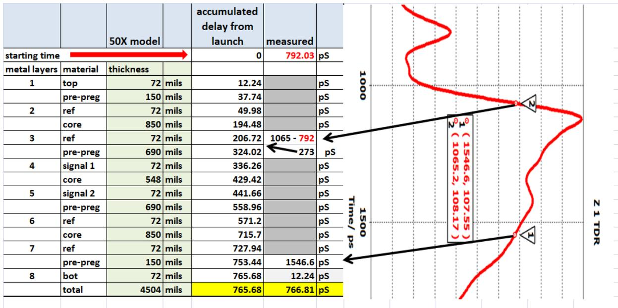
*Figure 23* Identify primary discontinuity by time positioning
