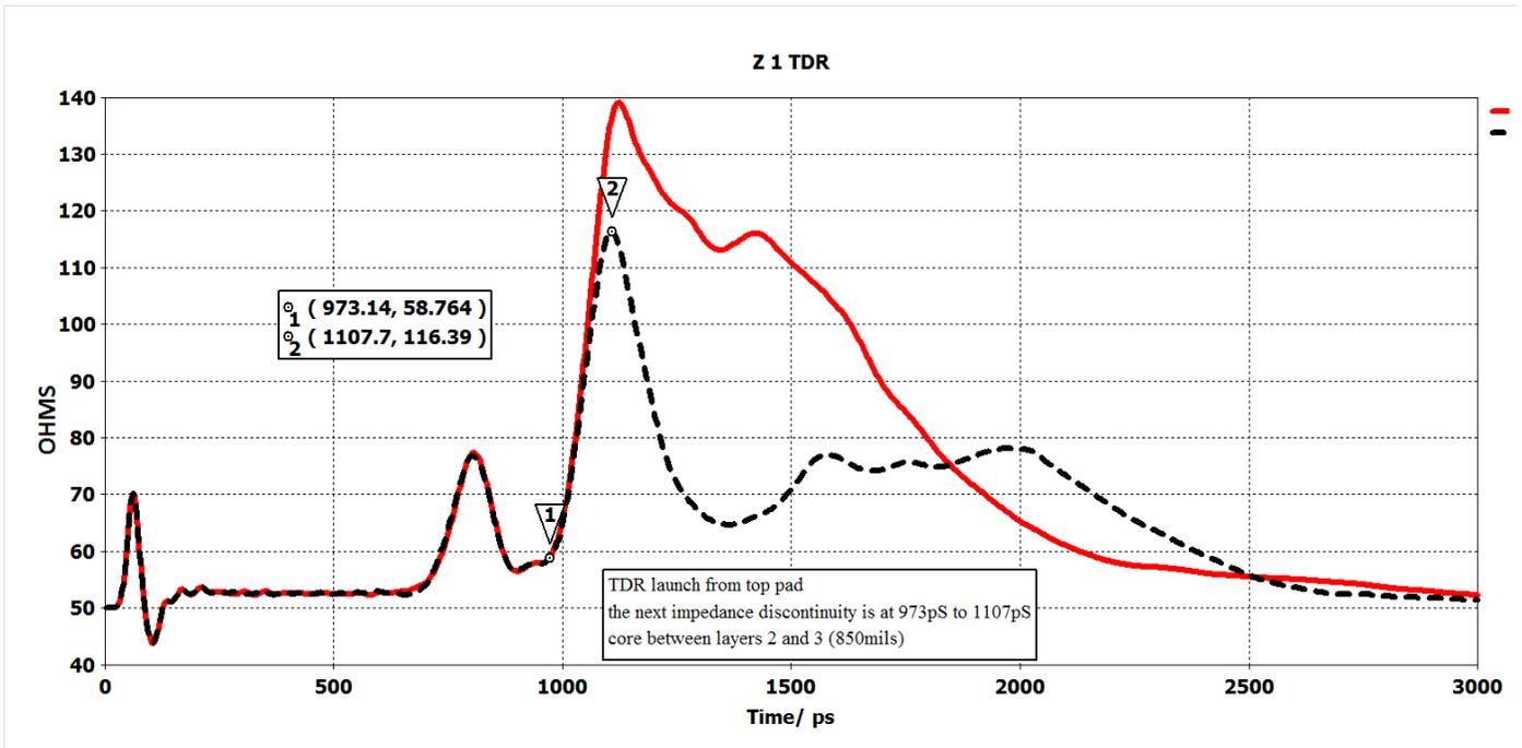
**Figure 24** Second major impedance discontinuity, Top pad launch, TDR riser time=30ps
