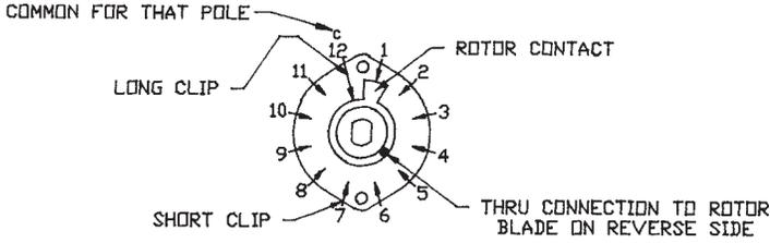
ALL DIAGRAMS ARE DRAWN AS VIEWED FROM THE KNOB END OF THE SWITCH, WITH THE LOCATING LUG IN THE 9 O'CLOCK POSITION AND THE SHAFT IN THE EXTREME COUNTER CLOCKWISE POSITION.
