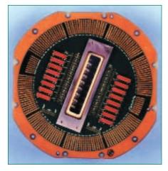
Figure 1. Probe cards for higher pin counts have to accommodate higher pad density where pad pitches are becoming finer and finer.
